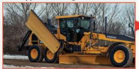
Preloaded Extension arm spring maintains blade stability in carry position.
