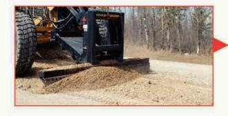
The Road Groomer attachment cuts washboards, ice, and removes rocks from road surface
