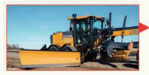
Blade has a 12' cutting edge, 30" intake and a 40" discharge.
